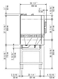
Cold Water inlet 1 (cleaning) = Cold Water Inlet 2 (steam generator) CWI2
